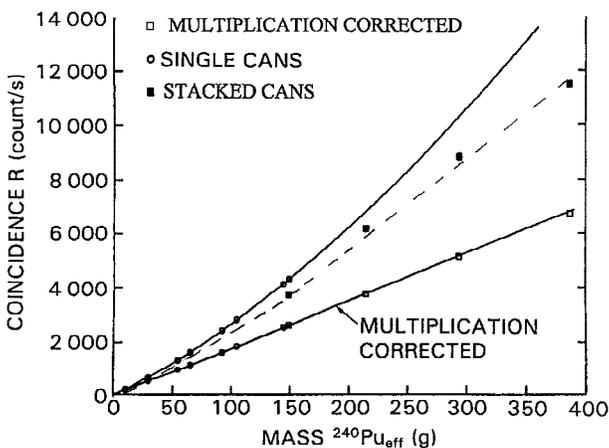
NOTE 1—Measured coincidence rate for two different measurement geometries (upper two curves) and multiplication corrected rate (bottom curve). Data for the curves was taken from Reference 20.
