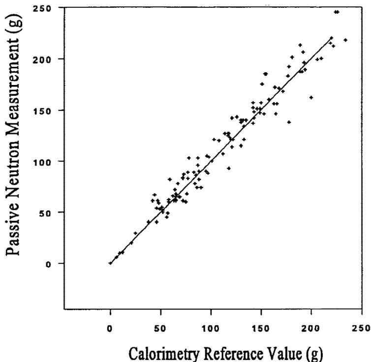
NOTE 1—The results of passive measurements of the plutonium content of small containers of scrap and waste are compared to the results of calorimetry and gamma-ray isotopic measurements. The containers were generated at a plutonium R&D facility in Los Alamos. The matrices do not contain hydrogen. The measurement uncertainties are dominated by bias rather than precision.
