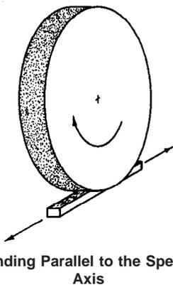
FIG. 5 Surface Grinding Parallel to the Specimen Longitudinal Axis
