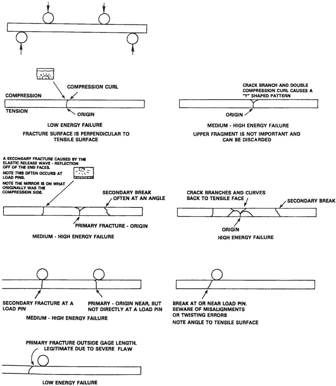
FIG. X2.1 Fracture Patterns
