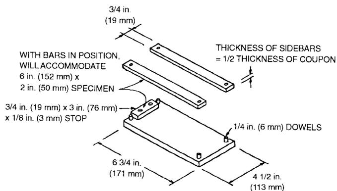
FIG. 1 Splitting Jig
