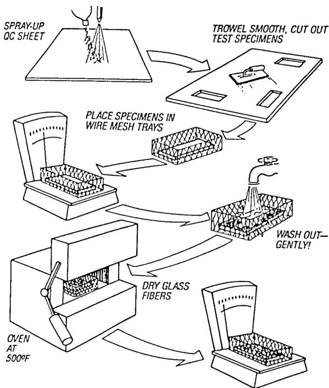
FIG. 2 Procedure for Determination of Glass Fiber Content
