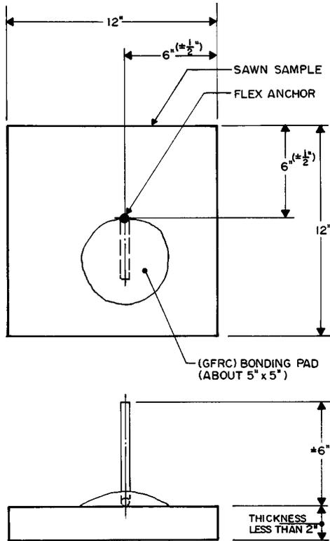
FIG. 4 Test Specimen
