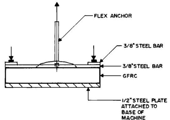
NOTE 1—Manufacture test specimens to keep flex anchor legs as vertical as possible. Support the legs if necessary during curing of the matrix.
