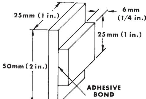
FIG. 1 Compressive Shear Specimen
