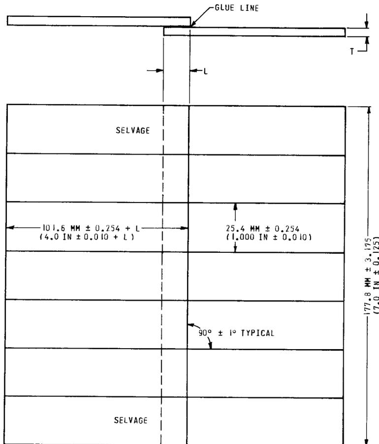
FIG. 1 Standard Test Panel and Specimen Configuration
