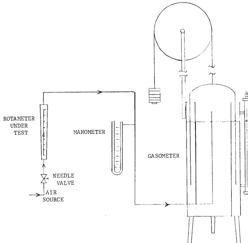
FIG. 2 Calibration Assembly Using Gasometer
