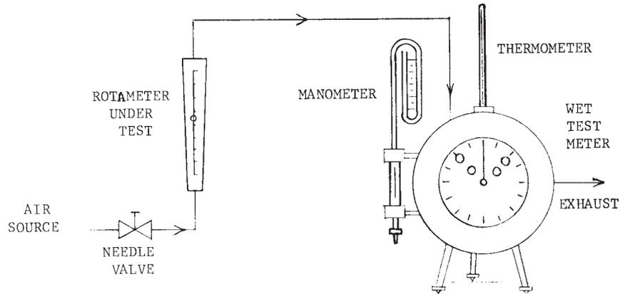
FIG. 1 Calibration Assembly Using Wet Test Meter
