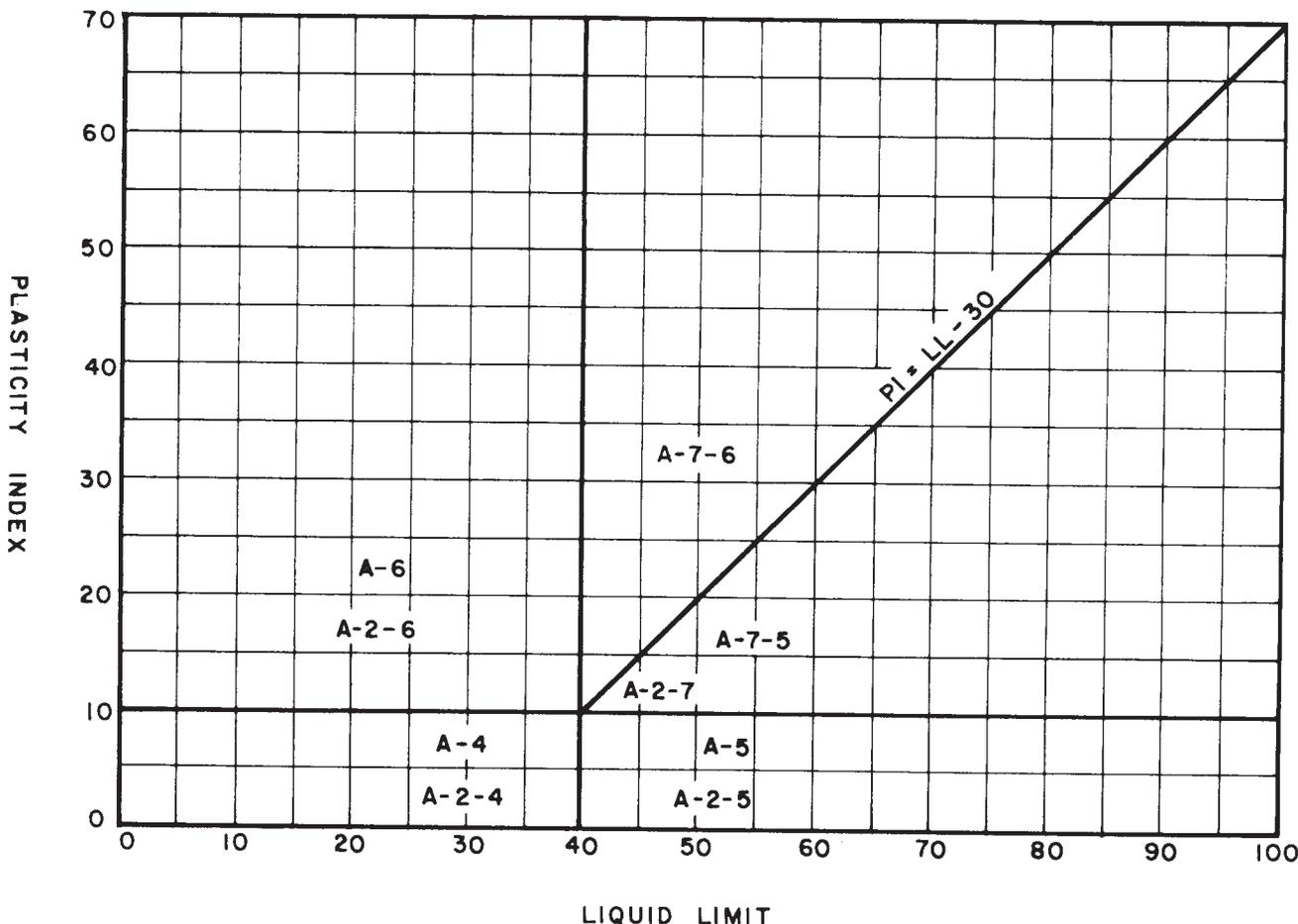
NOTE 1—A-2 soils contain less than 35 % finer than 200 sieve.
