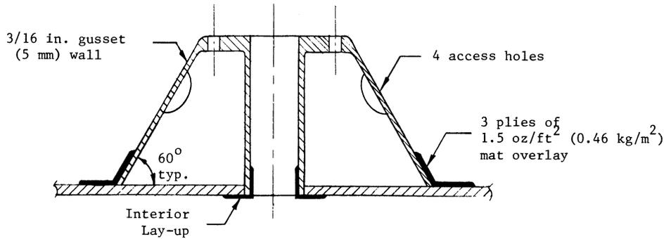
NOTE 1—This design does not require lay-up of nozzle neck to exterior of tank wall. Nozzle may be penetrating type or flush type as illustrated.
