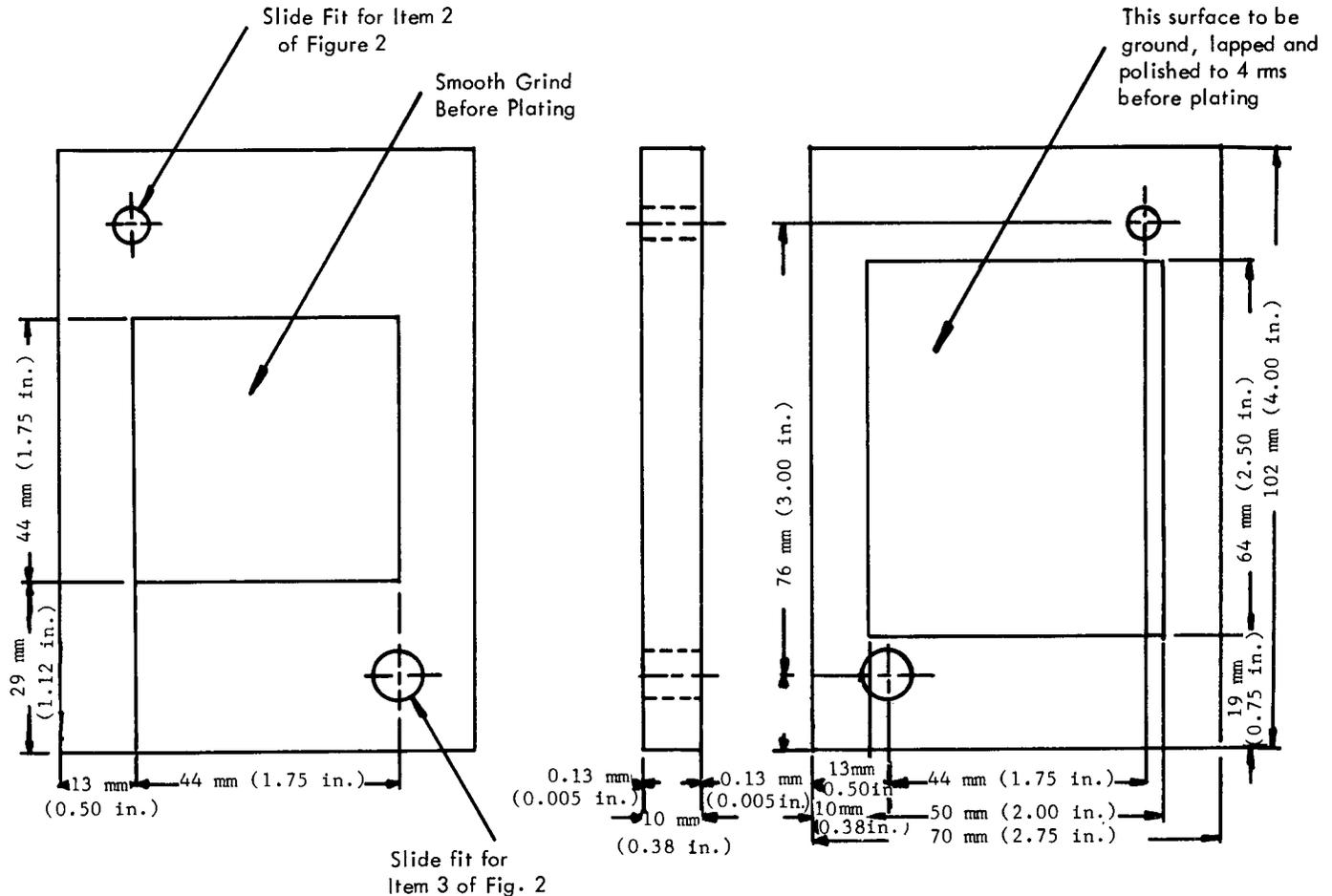
FIG. 1 Mold, Top Platen
