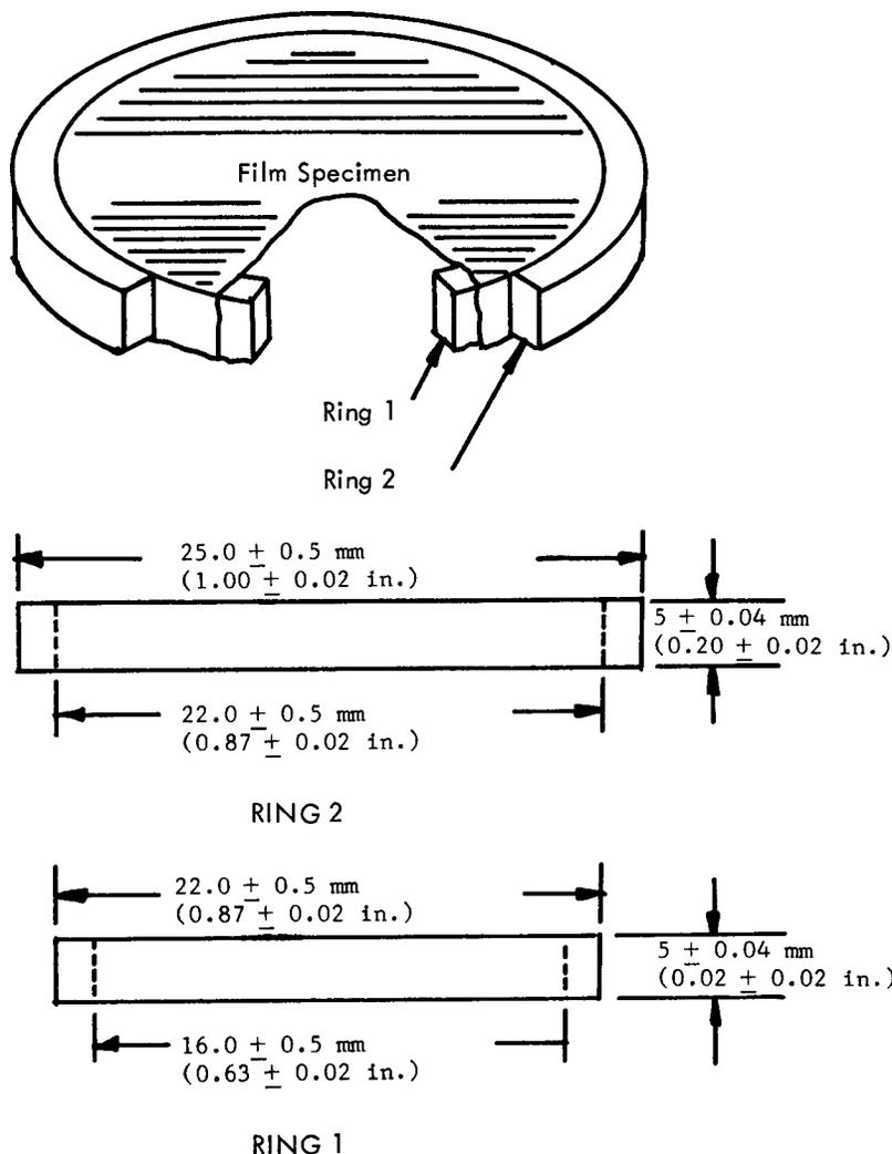
NOTE 1—Adjustments to the inside diameter of Ring 2 or outside diameter of Ring 1 may be necessary to obtain a snug fit of pressed film.
