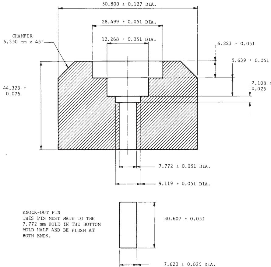
NOTE 1—Diameters are concentric. These two parts will be made of stainless steel. All dimensions are in millimetres.
