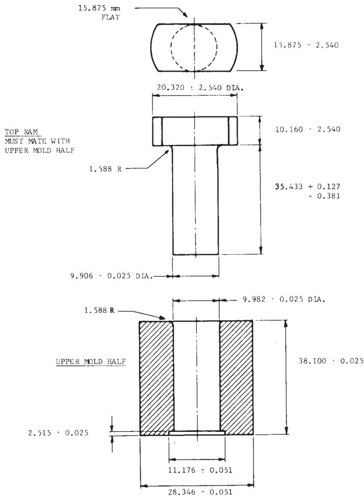
NOTE 1—Diameters are concentric. These two parts will be hardened tool steel and then ground to final dimensions. All dimensions are in millimetres.
