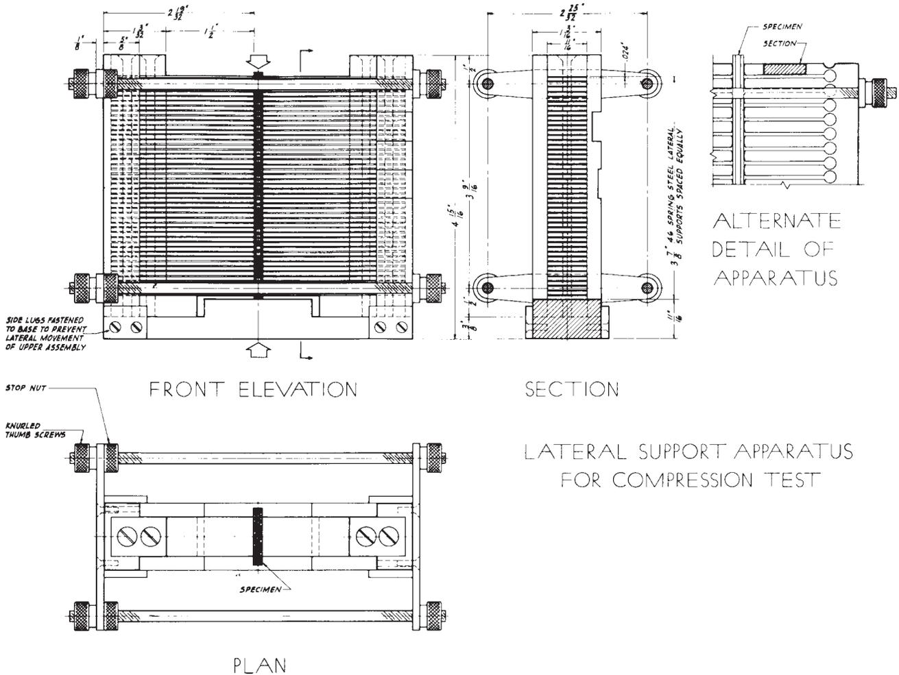
LATERAL SUPPORT APPARATUS FOR COMPRESSION TEST
