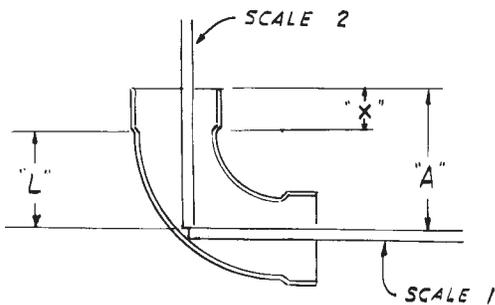
FIG. 1 Measurement for Calculation of Laying Length
