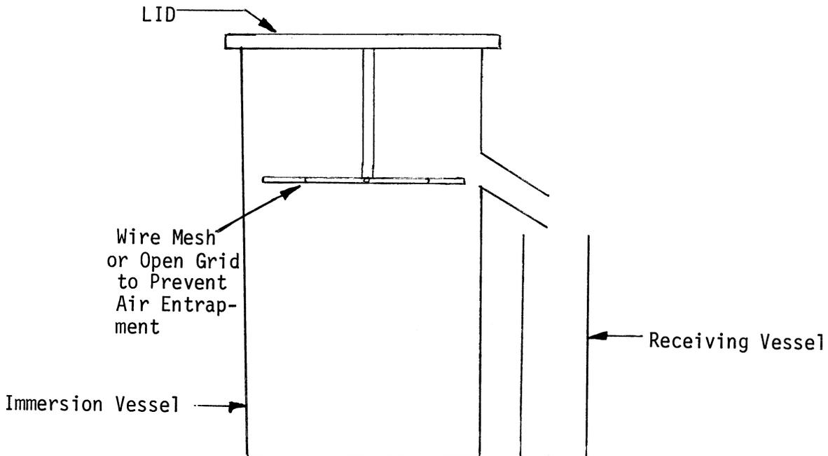
FIG. 1 Apparatus for Density Test Method B
