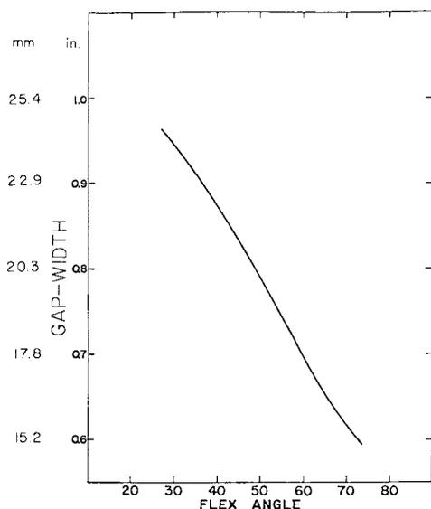
FIG. 6 Relationship Between Gap-Width and Flex Angle
