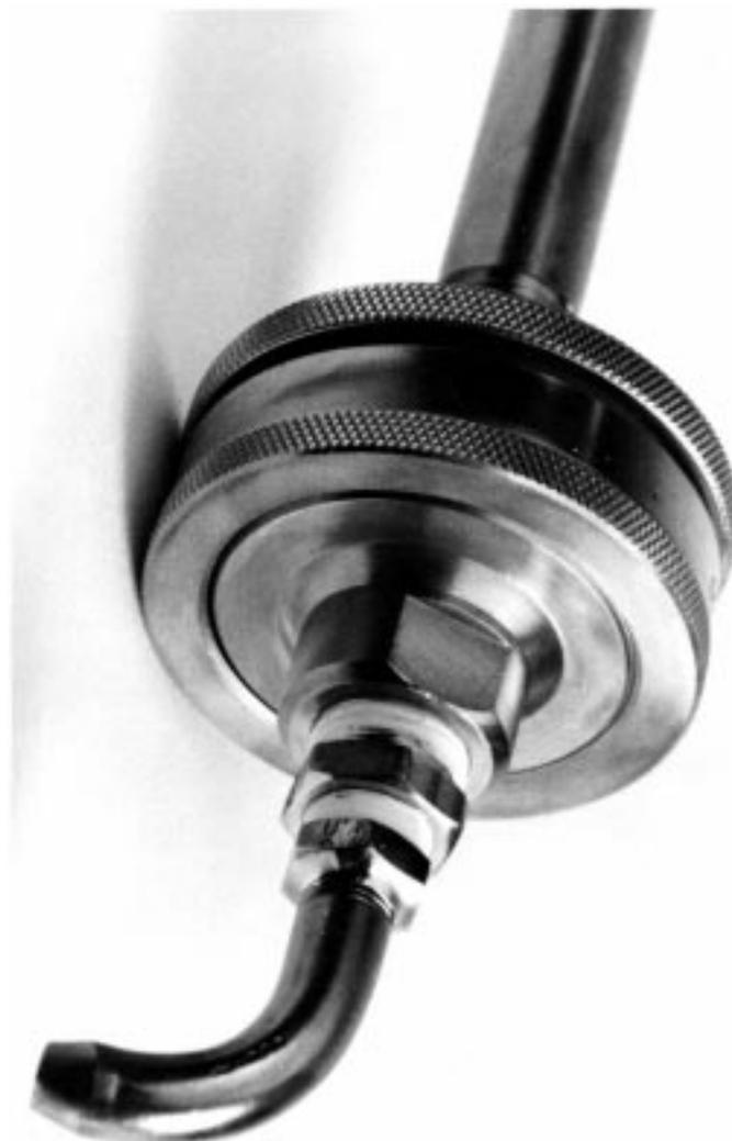
FIG. 6 Typical Holder for Flat, Round Filters
