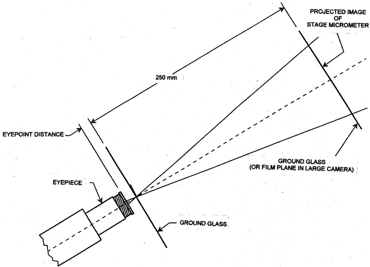
NOTE 1—A schematic diagram illustrating the procedure used to determine the magnification observed through the microscope eyepieces.
