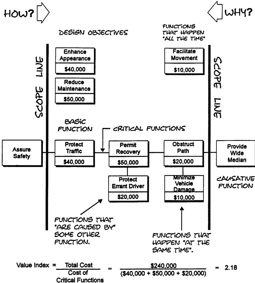
FIG. A1.2 Alternative Barrier Functions
