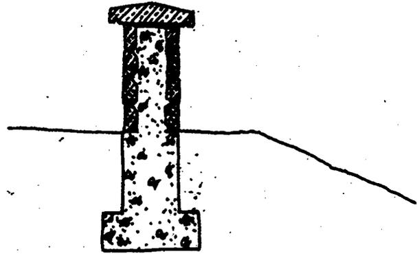
FIG. X1.2 Concrete Guardwall
