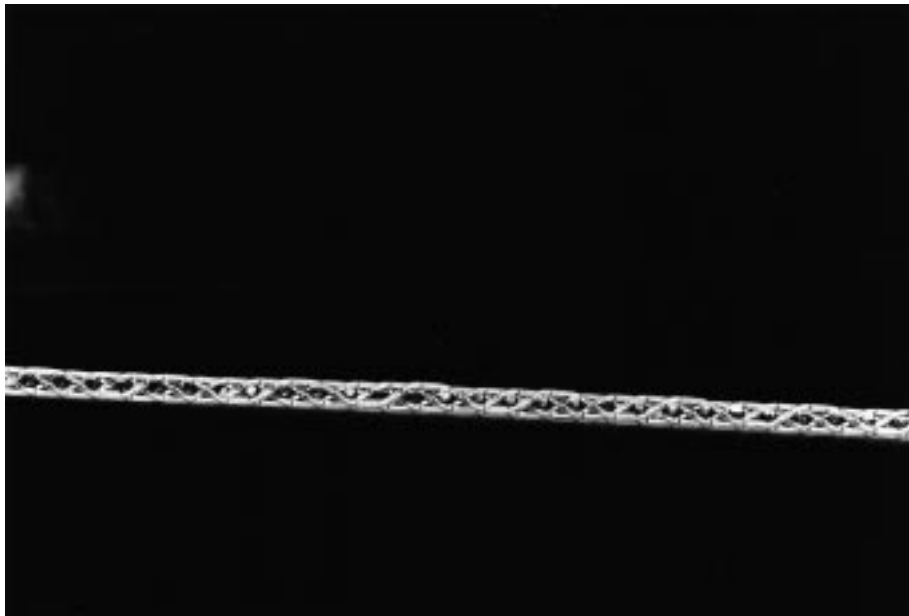
FIG. X1.2 Twilled Dutch Weave
