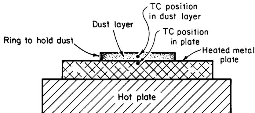
FIG. 1 Schematic of Hotplate Layer Ignition Apparatus
