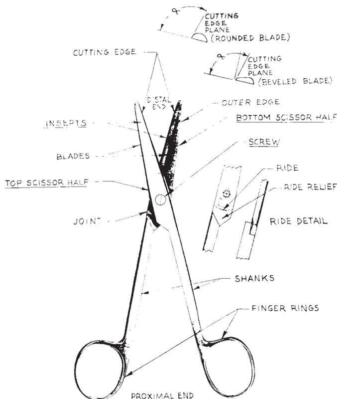
FIG. 1 Components of a Scissors (Inserted and Non-Inserted)
