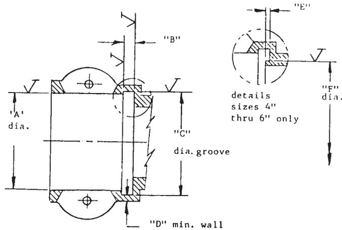
NOTE 1—Unidentified tolerances; fractional =  $\pm 1/64$  ( $\pm 0.4$ ), angular =  $\pm 2^\circ$  ( $\pm 0.035$  rad), decimal =  $\pm 0.005$  ( $\pm 0.127$ )
