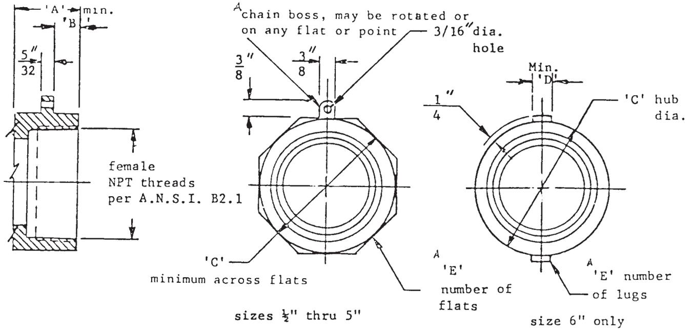
NOTE 1—<sup>A</sup> Chain boss to be provided at the manufacturer's discretion; number of flats or lugs provided are at the manufacturer's discretion. Unidentified tolerances; fractional  $\pm 1/32$  ( $\pm 0.8$ )
