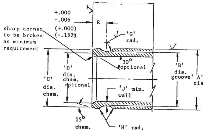
NOTE 1—Unidentified tolerances; fractional =  $\pm 1/64$  ( $\pm 0.4$ ), decimal =  $+0.000/-0.005$  ( $+0.000/-0.127$ ), angular =  $\pm 2^\circ$  ( $\pm 0.035$  rad)
