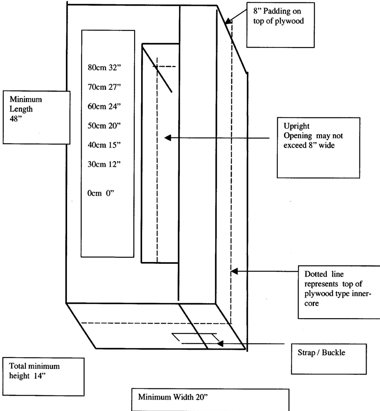
FIG. 7 Standard Base Padding With Depth Settings
