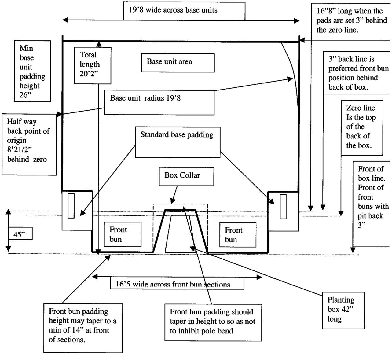
FIG. 2 Minimum Pole Vault Landing Systems Footprint
