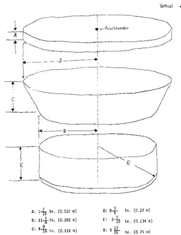
FIG. 8 Impacting Missile
