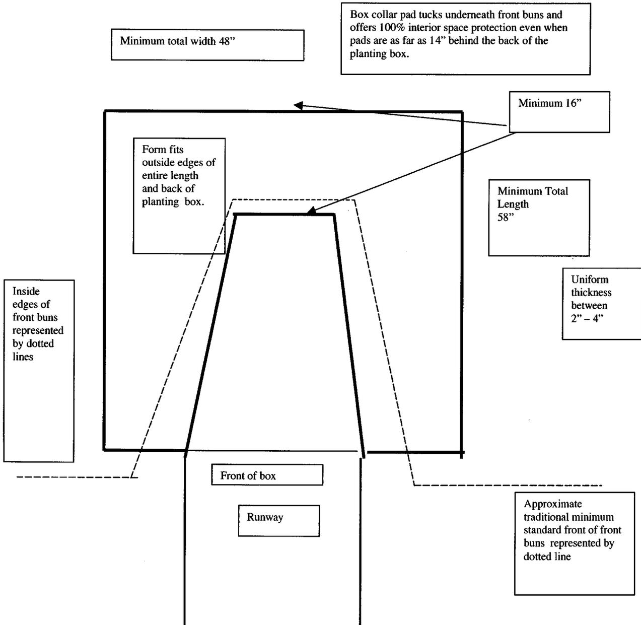
FIG. 3 Pole Vault Box Collar Minimum Specifications
