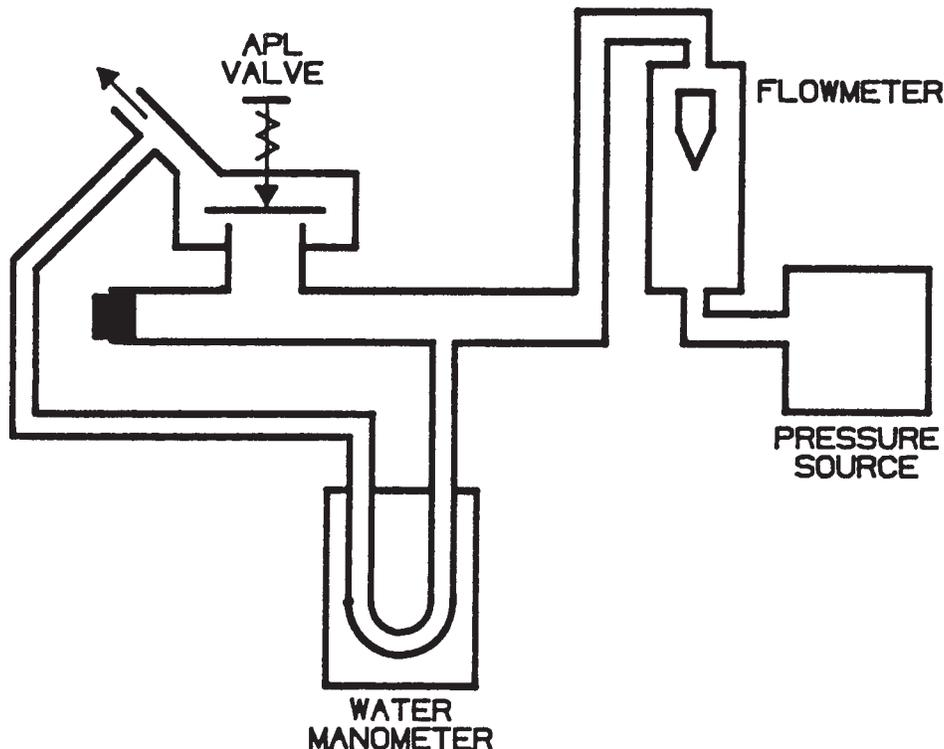
FIG. 4 Arrangement of Apparatus for Resistance Test
