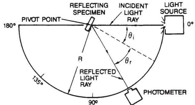
FIG. 1 Apparatus Set-Up
