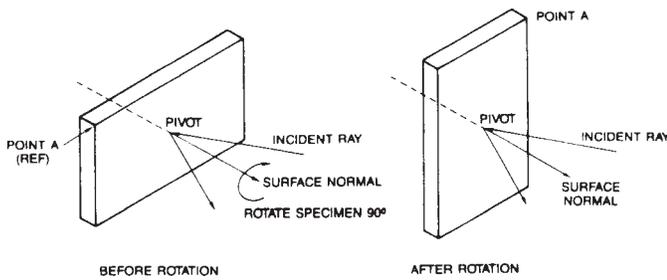
**FIG. 5 Rotation of Sample for Polarization Check**
