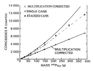
Note 1—Measured coincidence rate for two different measurement geometries (upper two curves) and multiplication corrected rate (bottom curve). Data for the curves was taken from Reference 20.
