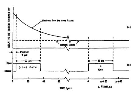
Note 1—Curve (a) is a simplified probability distribution showing the approximately exponential decay, as a function of time, for detecting a second neutron from a single fission event. The probability for detecting a random neutron is constant with time. Typical coincidence timing parameters are shown in (b).
