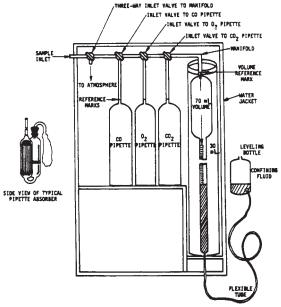
FIG. 5 Orsat Apparatus
