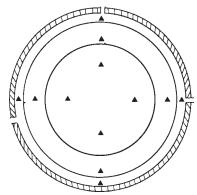
FIG. 8 Traverse Positions and Round Flue
