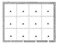
FIG. 7 Traverse Positions and Rectangular Flue
