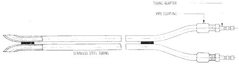
FIG. 3 Type 3 Pitot Tube (Special)
