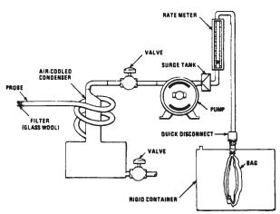
FIG. 4 Integrated Gas Sampling Train
