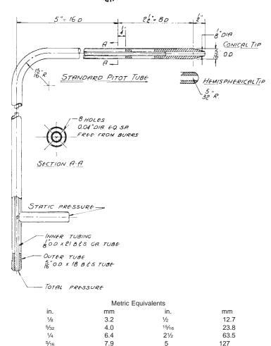
FIG. 2 Standard Pitot Tube Details
