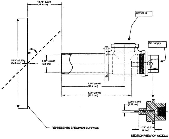
FIG. 1 Gravel Projecting Machine
