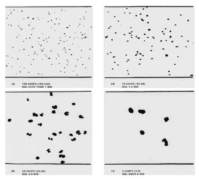
Note—Reprinted with permission from SAE EA-400 (c) 1985, Society of Automotive Engineers, Inc. FIG. 2 Representation of Chipping Ratings
