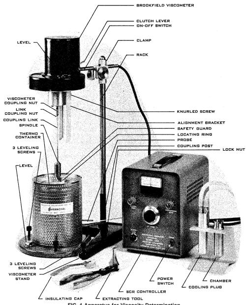
FIG. 1 Apparatus for Viscosity Determination
