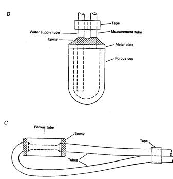
FIG. 3 Porous-Cup and Tube Designs
