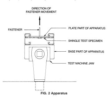
used, choose a scale in which the maximum pull-through force is at least 50 % of the full-scale reading.
