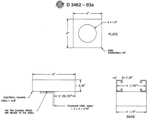
FIG. 1 Base and Plate Parts of Apparatus
