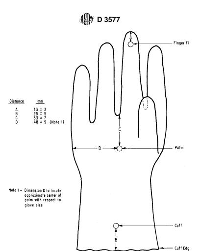
FIG. 1 Location of Thickness Measurements
