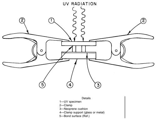
FIG. 3 Adhesive Joint Preparation
