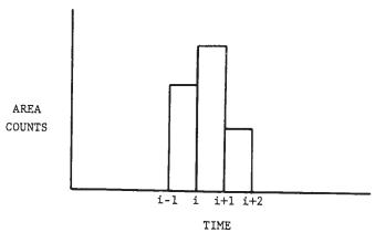
FIG. 3 Determination of Time to Peak Maxima
