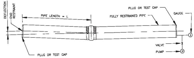
NOTE 1—Deflection (in.(mm)) = L(ft(m)) × offset (in./linear ft (mm/linear m)). See Table 2.
