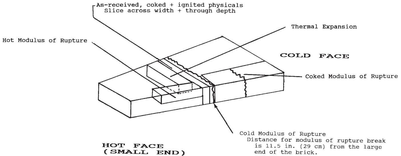
NOTE 1—For a 30-in. (76-cm) long brick the cold MOR is at 11½ in. (29 cm). All other brick sizes should be at the same relative distance or 38.3 % of the distance from the cold face, for example, for 18-in. (46-cm) long brick: 18 in. (46 cm) × 0.383 = 6.89 in. (17 cm) from the cold face. Physical sample must be taken out of the influence of the cold MOR break.
