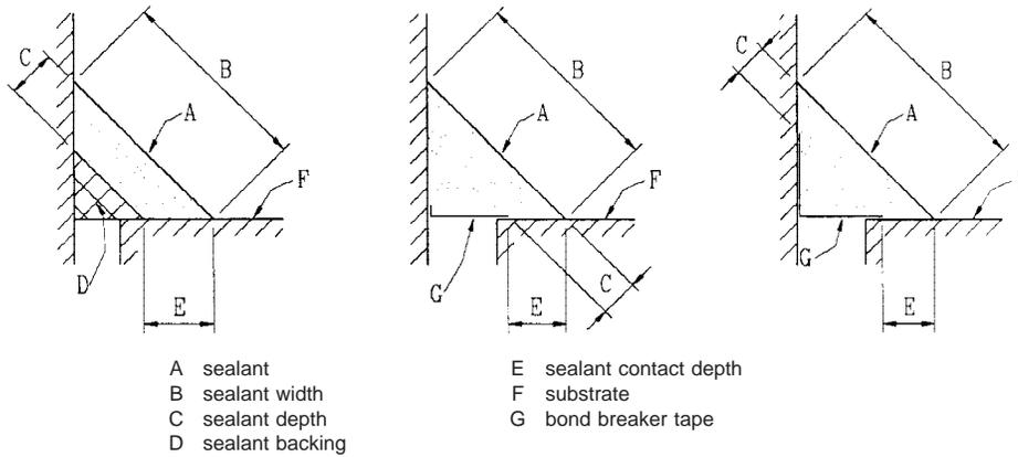
NOTE 1—The sealant surface can be tooled flat as indicated or concave or convex depending on an application's requirements.
