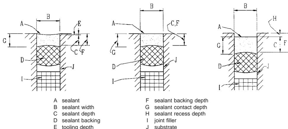
FIG. 4 Typical Butt Type Sealant Joint Cross-Sections
