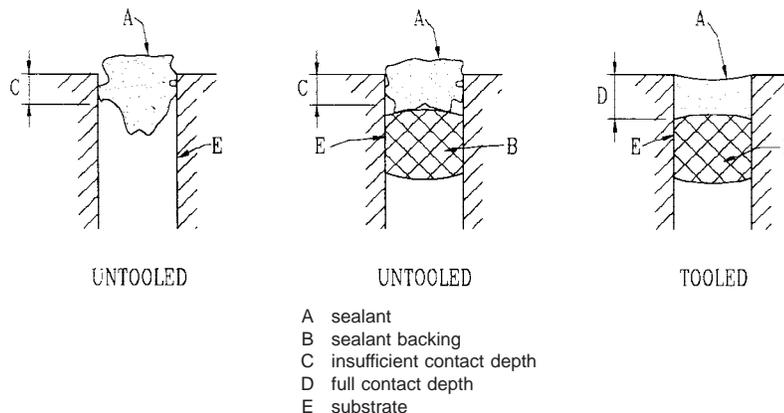
FIG. 10 Importance of Sealant Backing and Sealant Tooling
