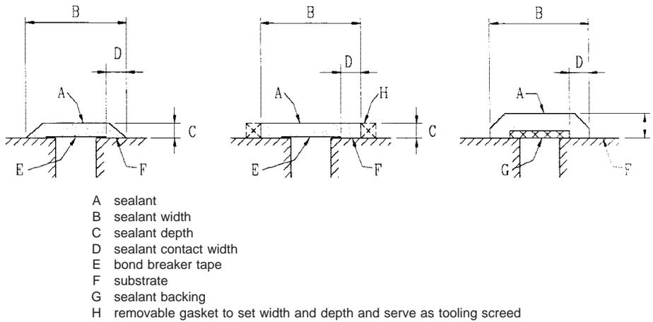
FIG. 6 Typical Liquid-Applied Bridge Sealant Joint Cross-Sections
