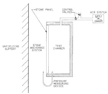
FIG. 1 General Arrangement of Testing Apparatus
