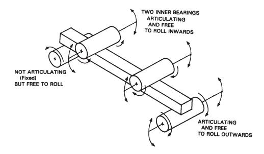
(b) FULLY-ARTICULATING. The two inner bearings are free to roll inwards, and they can independently articulate to match the specimen top surface. The two outer bearings are free to roll, and one bearing can articulate to match the specimen bottom surface.
