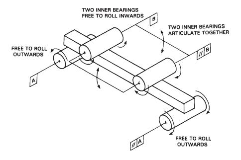
(a) SEMI-ARTICULATING. The two inner bearings are parallel to each other and the bearings are free to roll inwards. The two outer bearings are parallel to each other, and the bearings are free to roll outwards. The two inner bearings can articulate together as a pair to match the specimen top surface. (Alternatively, the two bottom bearings can articulate to match the bottom surface.)
