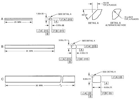
FIG. 4 Standard Test Specimens
