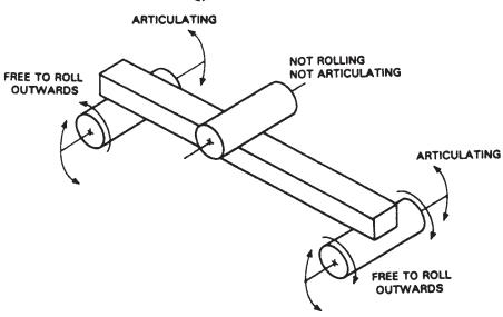
(c) FULLY-ARTICULATING (Alternative design) The two support bearings are free to roll outward. Both support bearings can articulate to match the specimen surface. The middle bearing does not roll and does not articulate.
