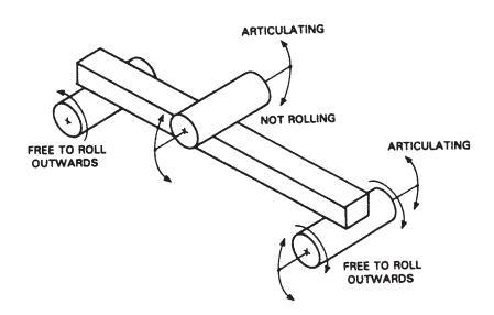
(b) FULLY-ARTICULATING The two support bearings are free to roll outward. One support bearing can articulate to match the specimen surface. The middle bearing does not roll, but it can articulate to match the specimen top surface.
