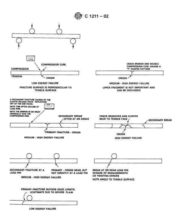
FIG. X2.1 Fracture Patterns
