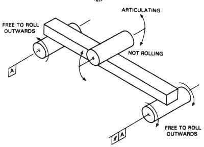
(a) SEMI-ARTICULATING. The two support bearings are parallel to each other and they are free to roll outward. The middle bearing does not roll, but it can articulate to match the specimen top surface.
