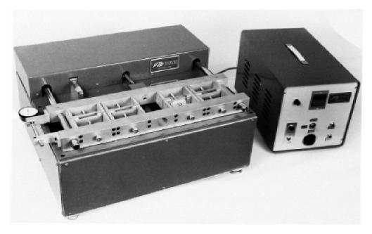
Note—Three-dimensional view of compression-extension machine with automatic control units shows four specimens ready for compression-extension cycling.
