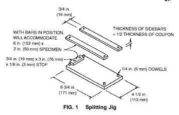
through the thickness of the coupon can be obtained by repeating the procedure on coupons slit into two halves through the thickness using the splitting jig as shown in Fig. 1. If this is done, the two halves should have approximately equal mass.
