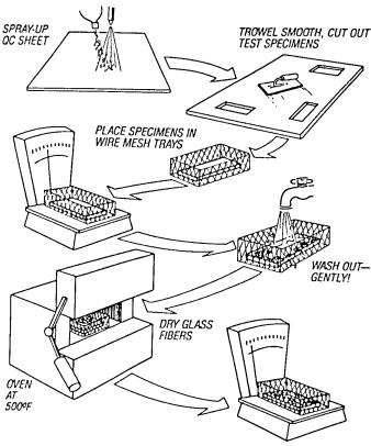
FIG. 2 Procedure for Determination of Glass Fiber Content
