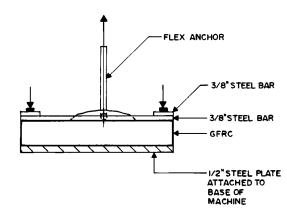
Note 1—Manufacture test specimens to keep flex anchor legs as vertical as possible. Support the legs if necessary during curing of the matrix.
