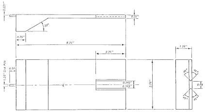
FIG. 10 Alignment Post for 6-in. [150-mm] Diameter Specimens
