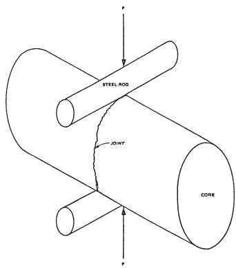
FIG. 1 Schematic of Loading Method
