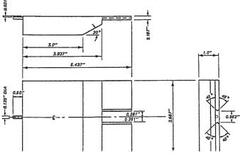
FIG. 9 Alignment Post for 4-in. [100-mm] Diameter Specimens
