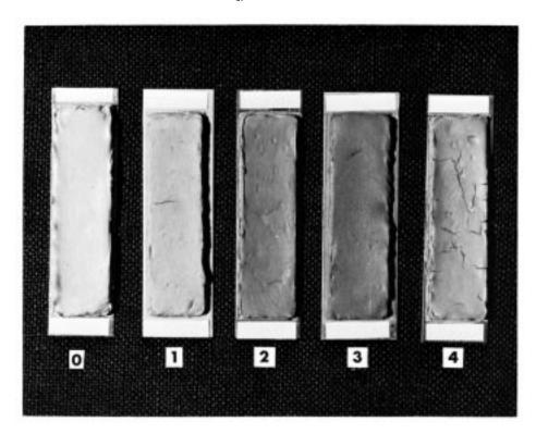
${\it Note} \ 1 {\it ---} Number \ 0 \ represents \ no \ cracking.$  FIG. 1 Examples of Cracking Obtainable in This Test
