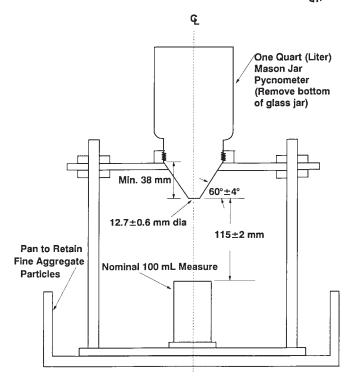
Section Through Center of Apparatus
