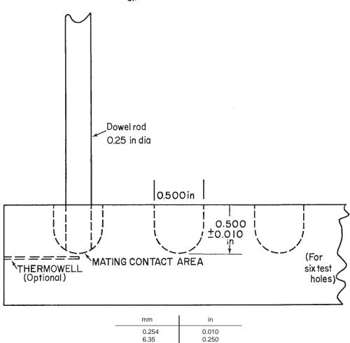
FIG. 1 Block, Drilled for Tests
