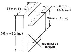
FIG. 1 Compressive Shear Specimen
