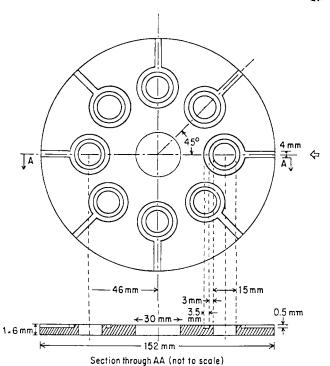
FIG. 1 Mold for Color Index Test
