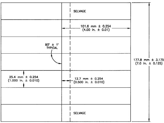
FIG. 2 Standard Test Panel
