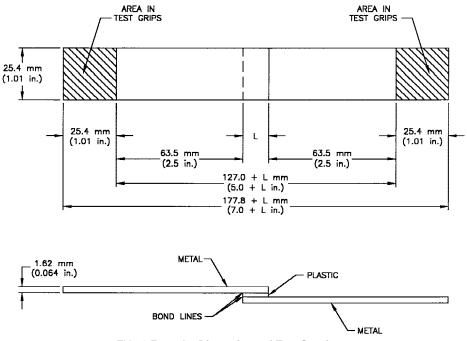
FIG. 1 Form A—Dimensions of Test Specimen
