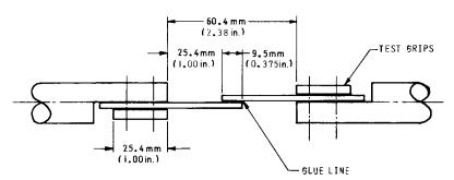
Note 1—Minimum specimen length in the grip 25.4 mm (1 in.). FIG. 1 Test Specimen
